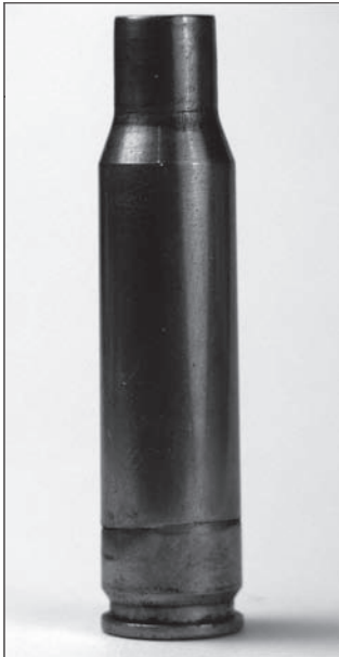
Case showing a split around the base just above the web.
