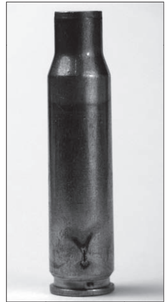
Old factory loaded case with split allowing gas to escape on firing.
