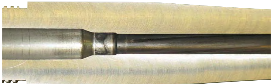
An eroded barrel will affect precision
