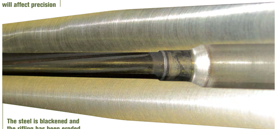
An eroded barrel will affect precision
