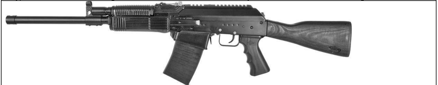
A typical box magazine shotgun – this version works on a gas bleed system
