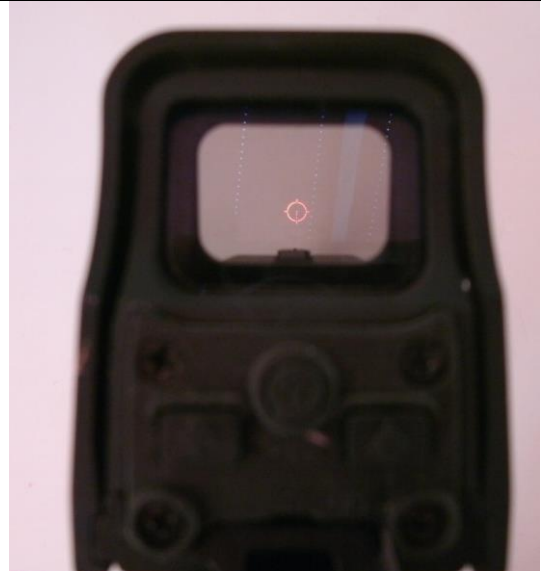
An LED within the sight projects an image of a circle or dot onto the glass lens and this is then zeroed to the point of impact. Brightness and size of the dot are sometimes adjustable.
