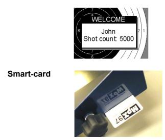
The Smart-card is inserted in the slot on the right side of the display. Make sure that the contact points are turned towards the back of the monitor.
