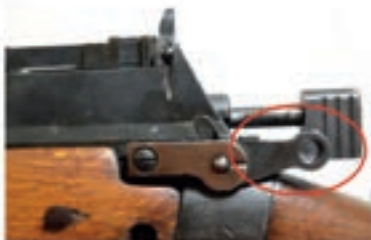
Safety Catch – applied. Rifle is cocked
