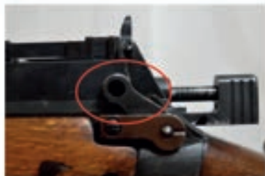
Safety Catch – not applied. Rifle is cocked
