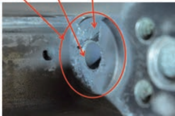
Ruger 10/22 chamber face showing fouling.
