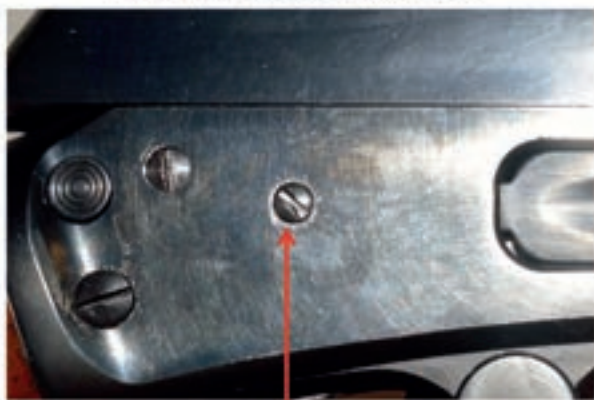
Damaged loading gate screw on a Marlin 1894. (Compare this to the two other screws visible in the picture.)
