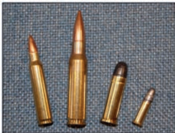
From left to right they are: 5.56mm – .308 Winchester – .38 Special – .22 LR
