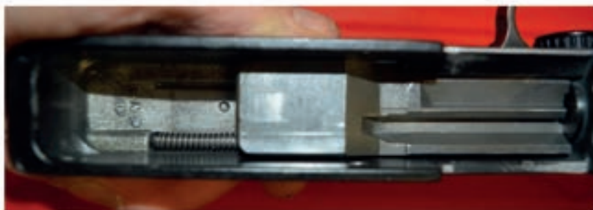
Cocking handle released, bolt in forward position.
