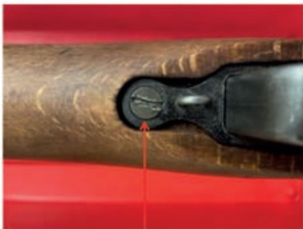
Damaged bedding screw on a No.4 Enfield
