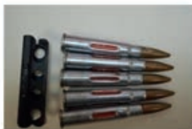
A charger clip and 5 drill rounds. Notice the up/down/up/down/up position of the cartridge rims.
