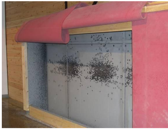
Figure 4 – LV bullet trap MS plate and Anti backslash curtain
