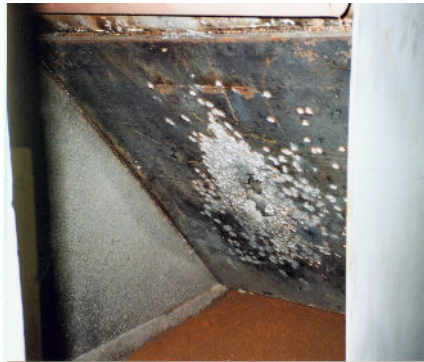
Figure 11 - .22" Penetrates Steel Plate
