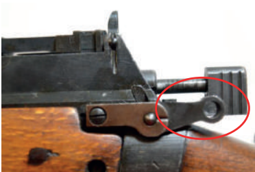
Safety Catch – applied. Rifle is cocked
