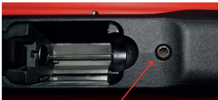
Action securing screw
