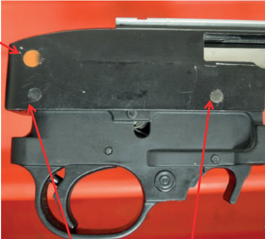
Trigger group locating pins
