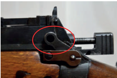
Safety Catch – not applied. Rifle is cocked
