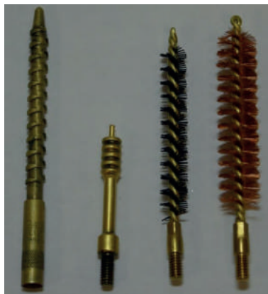
L to R: Wrap around brass jag (internal thread), spear-tipped brass jag (external thread), nylon brush (external thread), phosphor-bronze brush (external thread).
