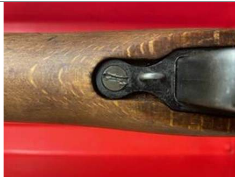
Damaged bedding screw on a No.4 Enfield
