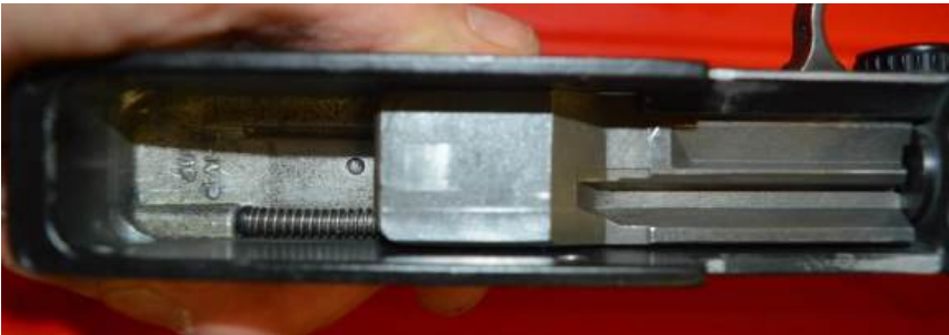
Cocking handle released, bolt in forward position.
