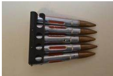
Drill rounds correctly placed into the charger.
