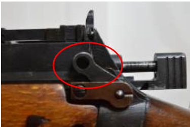
Safety Catch – not applied. Rifle is cocked
