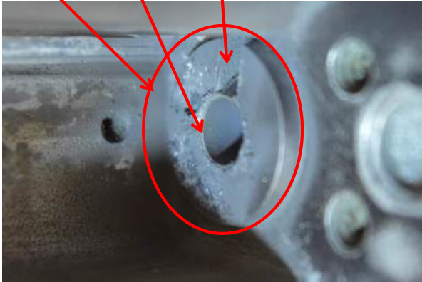
Ruger 10/22 chamber face showing fouling.
