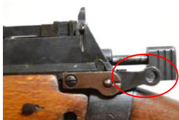
Safety Catch – applied. Rifle is cocked
