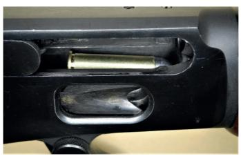
...when looked at from a different angle the cartridge nestling on top of the elevator couldn't be more obvious.
