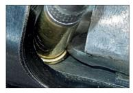
...and the rim is crushed by the front of the extractor. The cartridge explodes.
