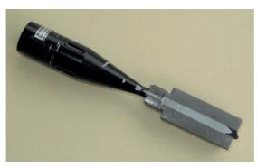
The mortal remains of a .22 barrel and the laser bore-sighter which the shooter forgot to remove before firing. In this instance no injury or other damage was caused. If this happens with a more powerful calibre there is an extremely high probability that the gun will blow up and cause serious injury
